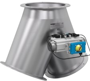
Example: Two-way valves with inlet collar 50°, symmetrical, construction DN > 300 mm with welded flanges, pneumatically operated with a rotary actuator
